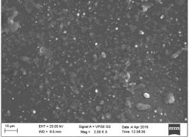
Figure 8 SEM image of 1:3 P:N Blend
